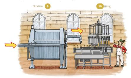
To complete the beer brewing process only one step remains. Step 10, *filling*. Depending on the brewery either cans or bottles are used to house the finished beer, until it finds the way to its eager consumer.<sup>12</sup>
