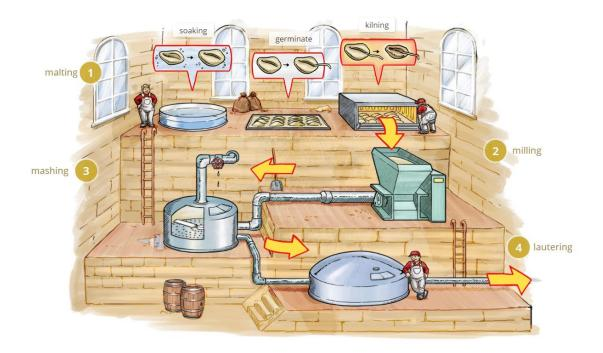
The first step of the brewing process is referred to as *malting*. Fresh barley gets soaked in water and put into germinating boxes which causes enzymes to form called amylase. This enzyme is essential because it allows for the starch to separate. At the perfect time, the germinating process is put to a halt and the malt is heated at 80° Celsius. This drying process is also called kilning and results in a malt with a slightly sweet taste.<sup>12</sup>
