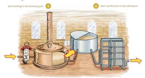
The sixth step is the *clarification* of wort. The wort continues on into a whirlpool that will rotate the liquid. The rotations cause any leftover trub to be centred in the middle of the pool, allowing for the clear wort to be tapped away from the outside. The clear wort is transported to a wort cooler, where it needs to be cooled to a temperature between 10° and 20° Celsius.<sup>12</sup>
